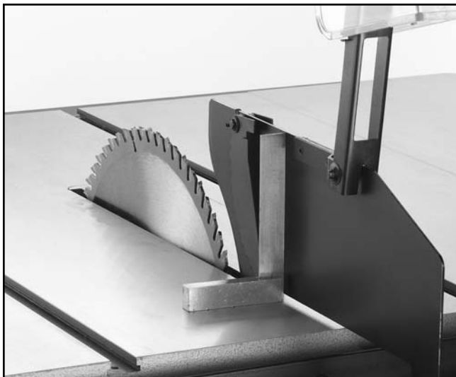
Figure 13. Guard assembly square to table.
